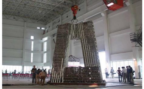
Figure 7. Shake table test model
