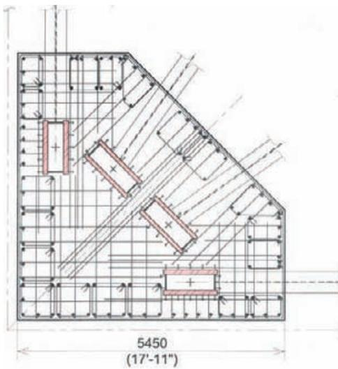
Figure 8. Plan of a corner mega-column.
