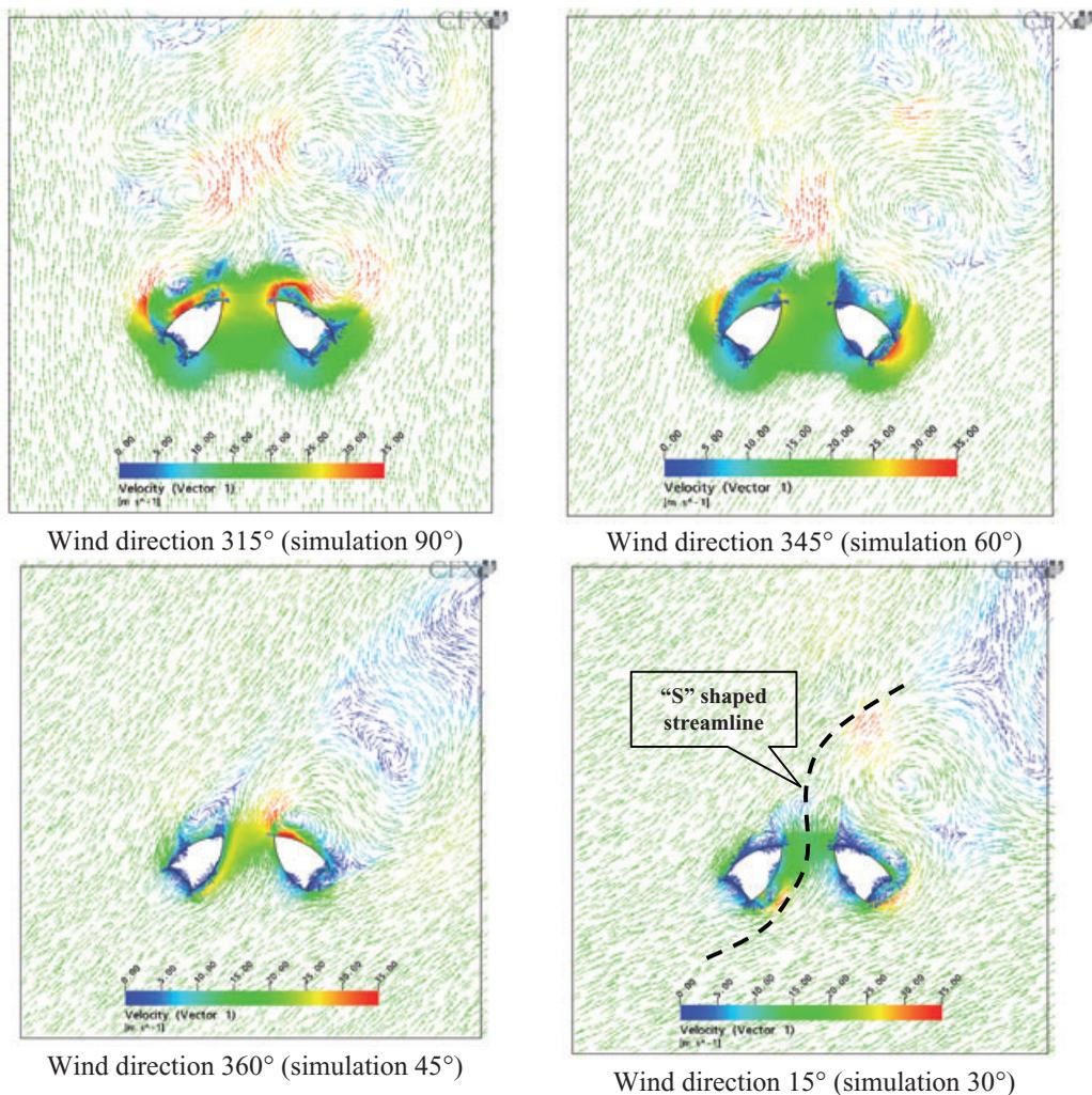
Figure 2. CFD Images by Ramboll, showing airflow patterns near towers, simulated at the level of the top turbine for different free, undisturbed wind incidence angles with respect to an 'x' axis (i.e., horizontal line connecting towers)
