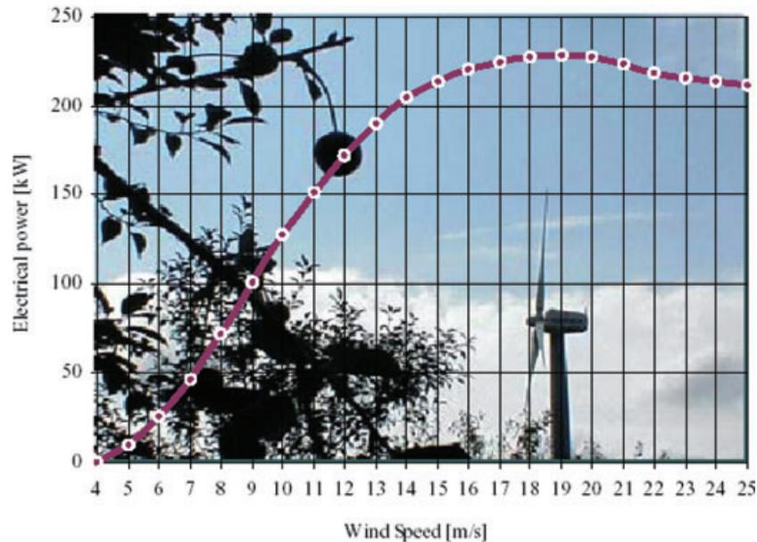
Figure 3. Electrical power versus wind speed
